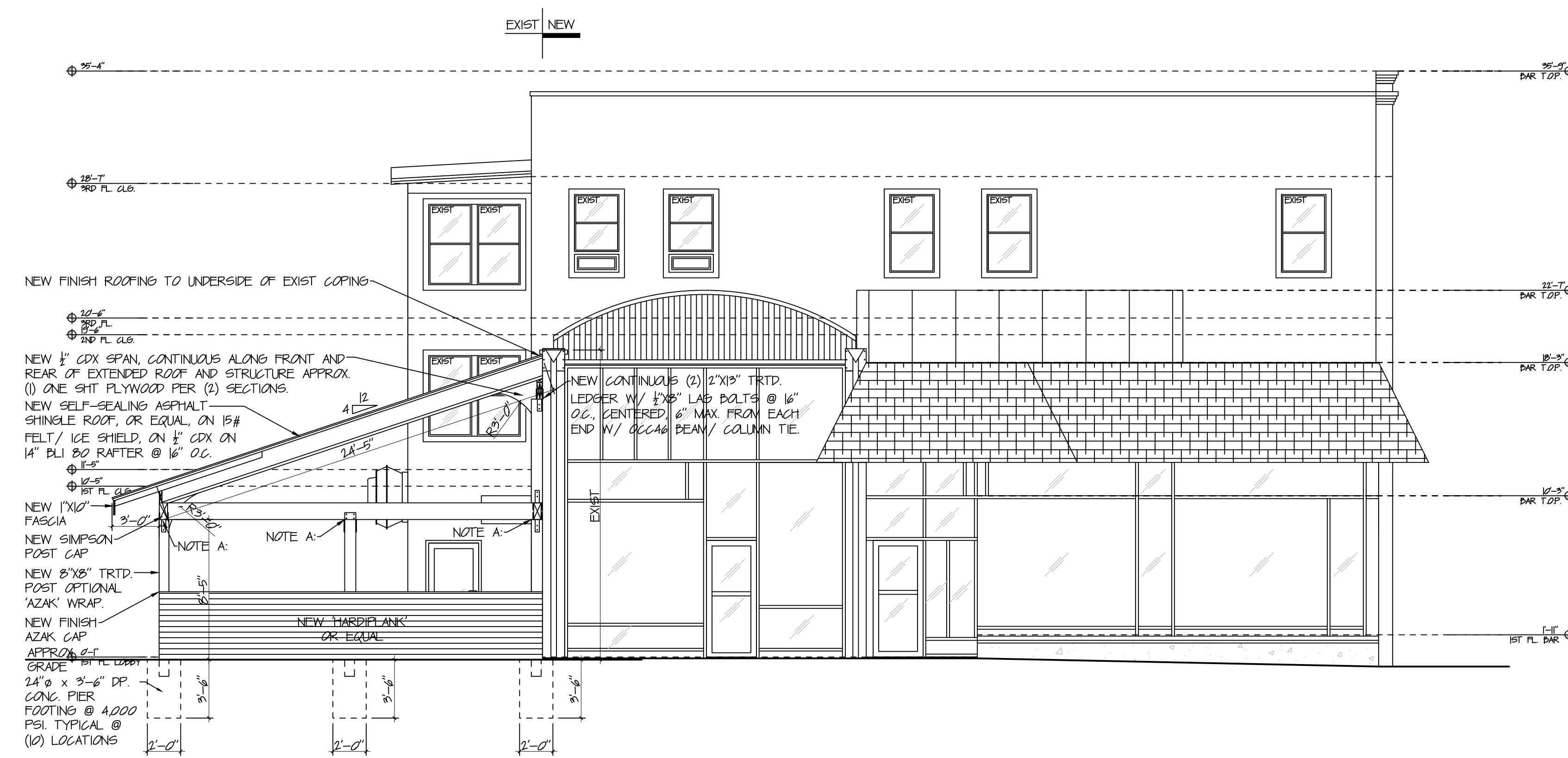
EXIST LEFT SIDE ELEVATION W/ CANOPY SCALE: 3/16" = 1'-0" NOTE A: NEW CONTINUOUS 5 1/2" x 11 3/4" DROP PARALLAM W/ SIMPSON CCG6PC BEAM COLUMN TIES, TYP. AT EACH LOCATION
